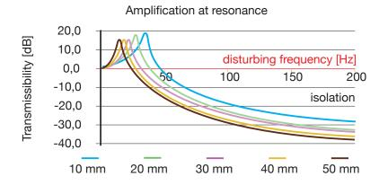
Read the Transmissibility by projecting a vertical line from the disturbing frequency to intercept the curve.
