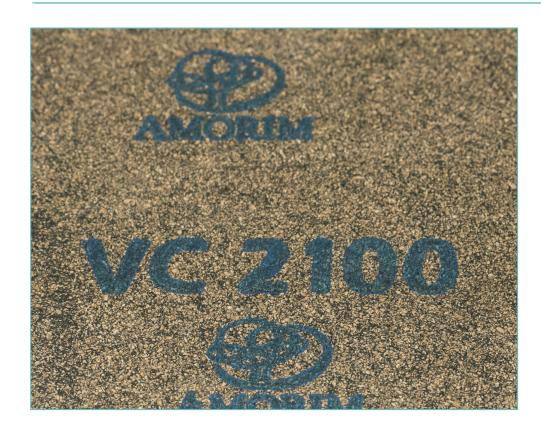
VC2100 Vibration Control material is an Engineered compound with Cork and Synthetic rubber. This product is suitable for vibration control applications in immersed in oil, such as internal vibration control pads in extreme industrial environments where the presence of oils or other chemicals are present.
