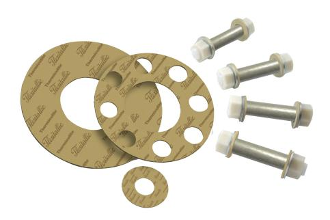
The Flexitallic I-Flex High Pressure Fire-Safe (FS-HP) Flange Isolating Set is comprised of a fire safe insulating gasket, insulating sleeves, insulating washers and metal backing washers.
