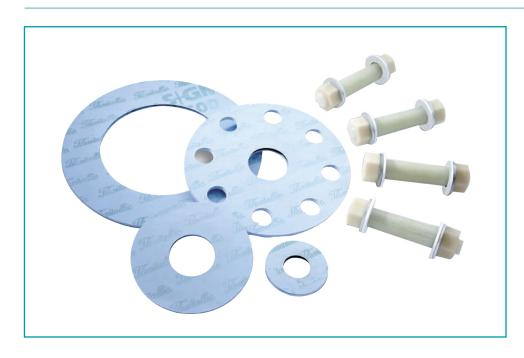
The SIGMA® 500 material is suitable for sealing all chemicals across the whole pH range (0-14) with the exception of molten alkali metals, fluorine gas or hydrogen fluoride.
