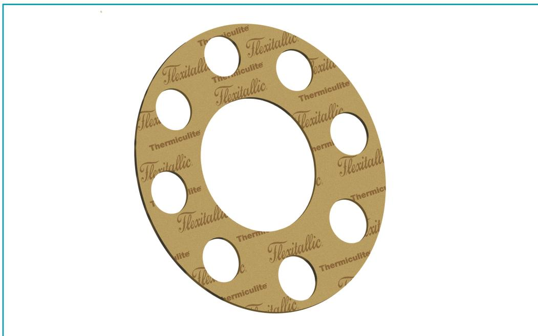
Thermiculite® 714 is an acid resistant calendered sheet sealing material reinforced with a blend of organic and inorganic fibres and bound in a specially formulated synthetic rubber binder matrix
