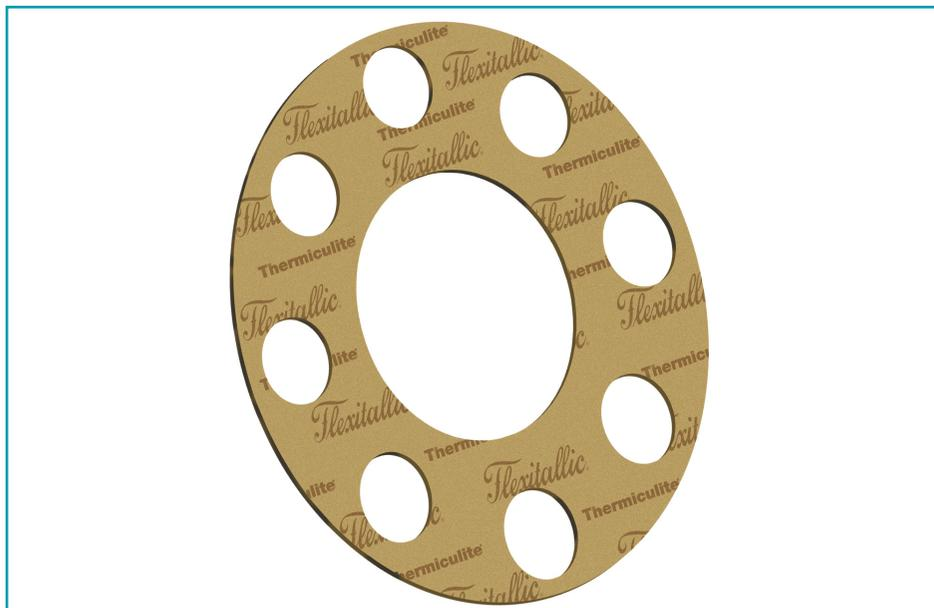
Thermiculite® 815 is a high temperature, chemical resistant sheet sealing material comprising exfoliated vermiculite reinforced with a tanged stainless steel core.
