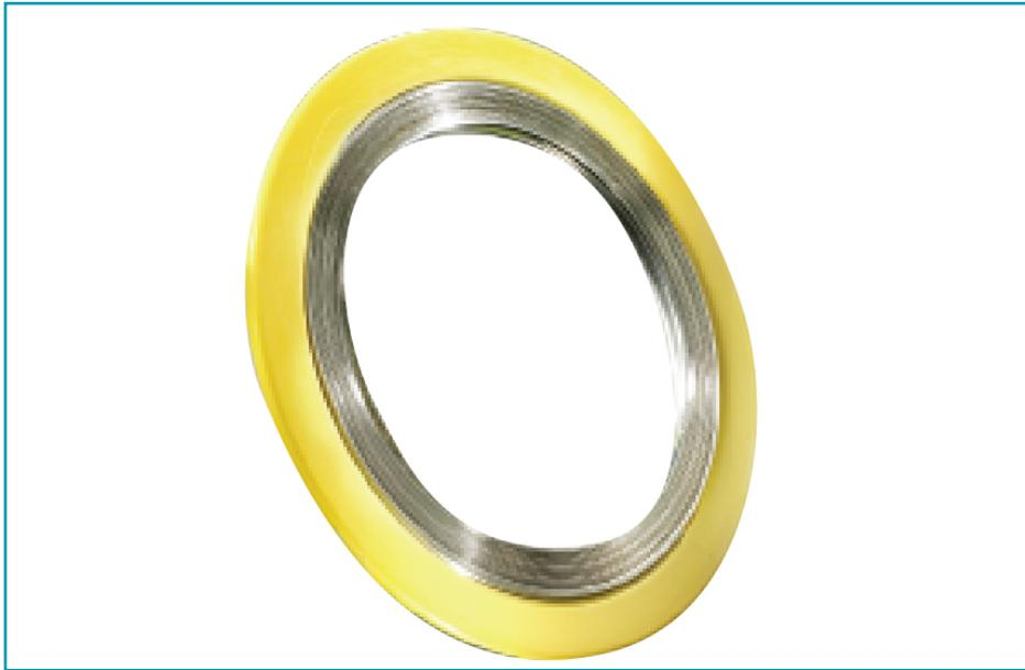
Flexitallic 835 is a critical service gasket designed for use in applications involving high temperatures and/or aggressive chemical media. It is comprised of a spirally wound sealing element composed of a metal winding wire in combination with a vermiculite based filler material.
