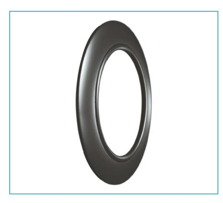
This gasket consists of a steel ring which is completely enclosed in rubber. It is suitable for drinking / cooling water, acids and alkalis, up to 40 bar. Dimensionally stable, large sizes easy to assemble, application general pipe construction.
